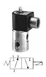
3-way Normally closed Port identification: 1-pressure/2-cylinder/3-exhaust
