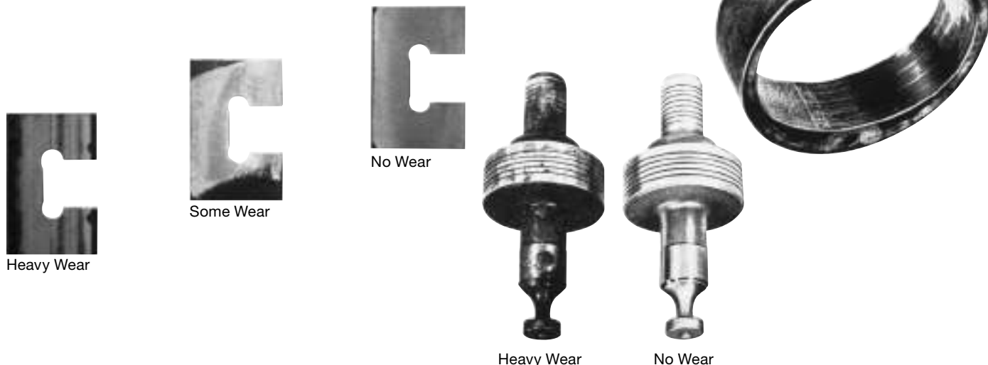
Figure 1. Typical Examples of Wear Due to Contamination
