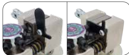
a tube-setting tab to ensure proper placement in the dies
