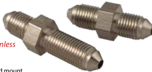
BQ292 -3 JIC Union BQ292SS Stainless version 3/8-24 UNF, 7/16" hex 30.7mm overall length
