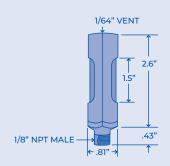
Sights are sized to fit existing or readily available fittings. Heavy duty material is used through (black oxide steel). Sights measure .81" wide by 2.6" high (male) or 2.17" high (female).
